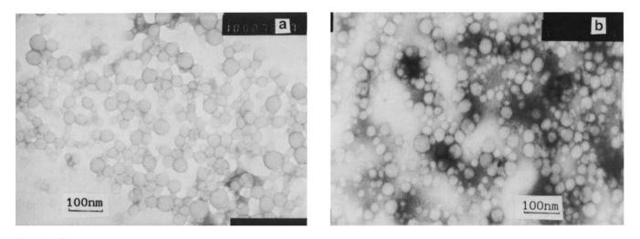
Figure 2 Transmission electron micrographs of polystyrene obtained from microemulsions using (a) BCa and (b) Ce
