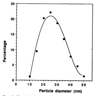
Figure 3 The size distribution of polystyrene particles obtained from the BCa microemulsion
