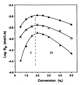
Figure 1 Effect of styrene concentration on polymerization using 0.6 mM KPS and carbitol cosurfactant at 50°C: ( $\triangle$ ) 2% styrene; ( $\Box$ ) 4% styrene; ( $\bigcirc$ ) 5.5% styrene
